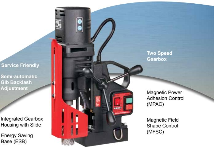
The PRO 51 is equipped with an electromagnetic energy saving base (ESB) which uses only 50% of the power when the motor is not under load, and a magnetic field shape control system (MFSC) which provides maximum holding power on thin material. A magnetic power adhesion control module (MPAC) detects an adequate adhesive force of electromagnetic base for safe operation.
