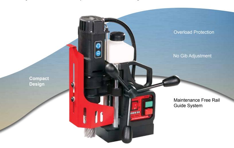
The PRO 36 is equipped with an electromagnetic energy saving base (ESB) which uses only 50% of the power when the motor is not under load, and a magnetic field shape control system (MFSC) which provides maximum holding power on thin material. A magnetic power adhesion control module (MPAC) detects adequate adhesive force of electromagnetic base for safe operation.
