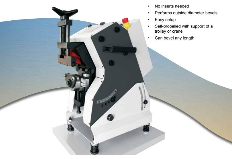
The beveling angle can vary from 22.5°, 30°, 37.5°, 45° and 52.5° by simply changing the working angle on the machine. Angle changing can be done rapidly and precisely with the locking preset scale on the side of the machine. There are no roller supports or attachments to change. The machine can be used in a stationary manner by hand feeding smaller parts or can be equipped with an optional height adjustable cart for traveling the length of large plates.
