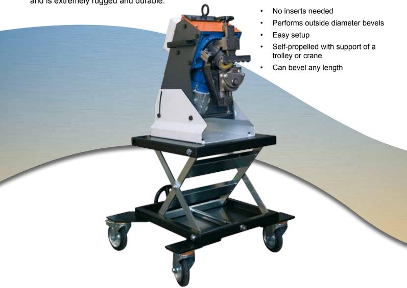
The beveling angle can vary from 22.5°, 30°, 37.5° and 45° by simply replacing the roller group. The machine can be used in a stationary manner by hand feeding smaller parts or can be equipped with an optional height adjustable cart for traveling the length of large plates.
